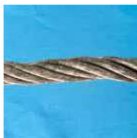
Reduction in wire rope diameter (hollowstand)
