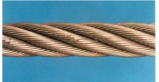
Broken wires on the surface
