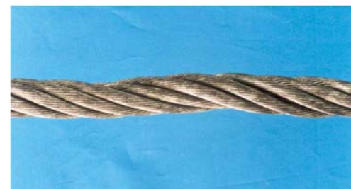
Localised reduction in the wire rope diameter (hollow strands)
