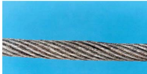
Localised increase in the wire rope diameter due to the core extruding
