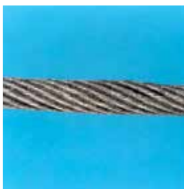
Increase in diameter due to the extrusion of the core
