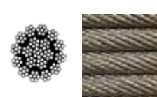
19x7 WSC ROTATION RESISTANT GALVANIZED WIRE ROPE Ø12mm (Ø 0.47in)
