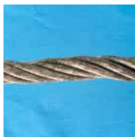
Reduction in wire rope diameter (hollowstand)
